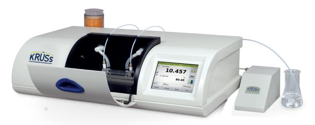
Semi-automatic sample supply with P8000-TF and peristaltic pump DS7070
